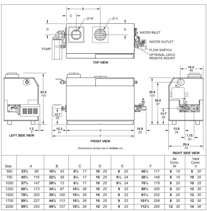
Figure 2. Dimensional Data (pump-mounted models).
